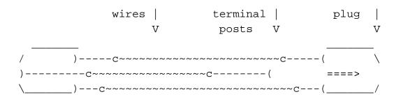
I hope this picture helps. It's not difficult. By the way, you don't have to solder if you really don't want to. You can find plugs which have screws rather than solder locations. You can make the wire without having to solder, but you'll probably lose the surety of the better connections made through soldering.
